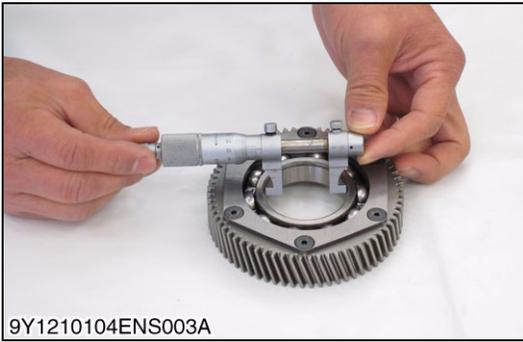
**Oil Clearance between Idle Gear Shaft 1, 2 and Idle Gear 1, 2 Bearing**
