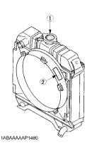
① Part No.19077-8724-1 or 16667-8724-1 (55mm in diameter) (37mm in diameter)
